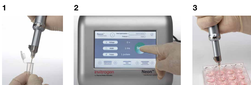
Figure 9.7. Simple 3-step transfection procedure. 1. Load mix of harvested cells and molecules to be delivered (e.g., DNA, RNA, protein) into the Neon system pipette tip. 2. Plug the pipette into position in the Neon transfection device, select your protocol, and press Start. 3. Unplug the pipette and transfer your transfected cells into a tissue culture vessel.
